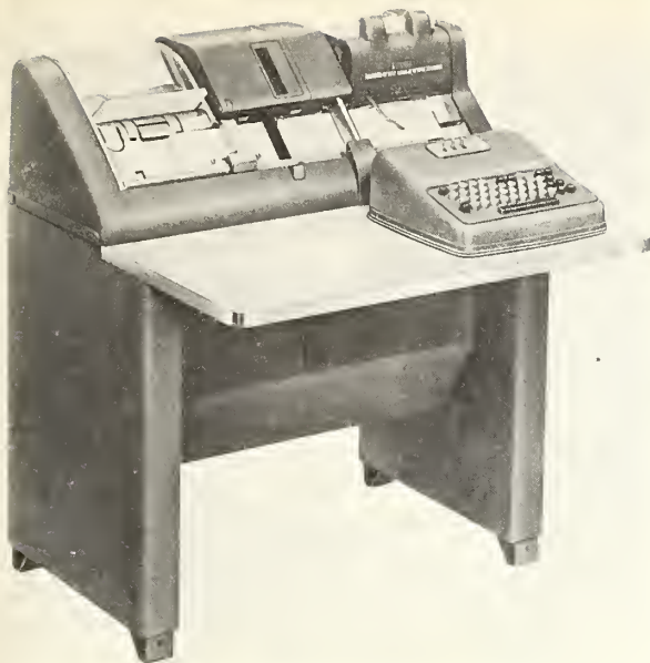
Figure 5.--A card punch used for recording alphabetic, numerical, and special character data into tabulating machine cards.
